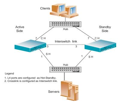
Figure 11-10 Hot-Standby Configuration
